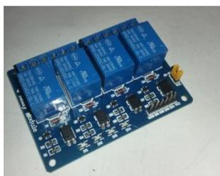
**Gambar 2. Relay 4 Channel**
