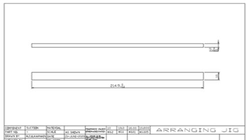
**Gambar 5. Production drawing JIG (Stick Frame bagian bawah)**
