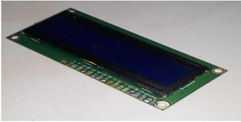
**Gambar 4. (Liquid crystal display) LCD**
