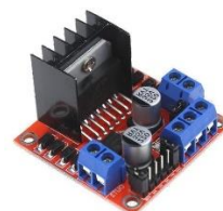
Gambar 5. Motor Driver L298N Sumber: (Data Penelitian, 2022)
