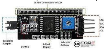
Gambar 5 Inter Integrated Circuit (I2C)
