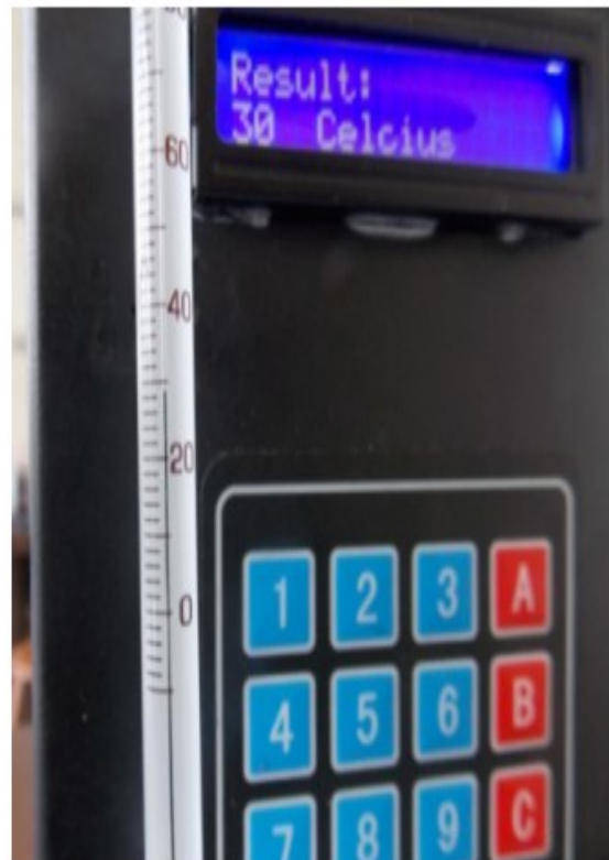
Figure 2. Test the detector with an analog room thermometer
