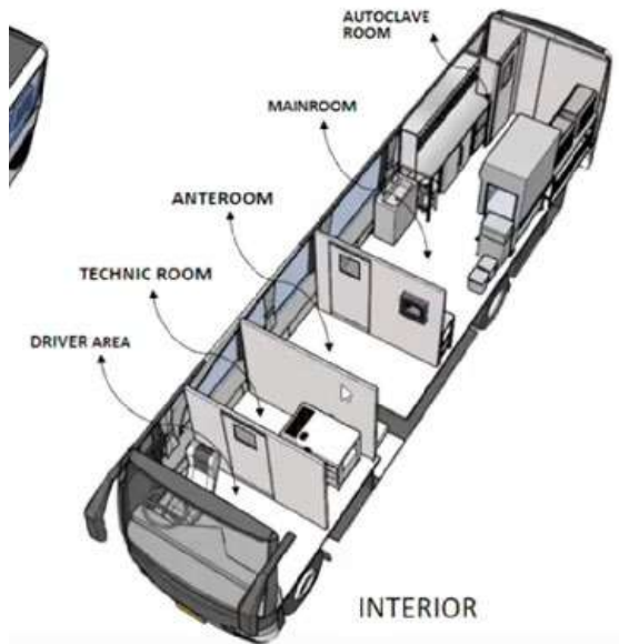
Gambar 5. Render gambar Mobile Lab BSL-2 Gen3, Tipe Bus
