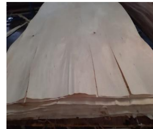
Gambar 5. Dokumentasi Defect Core Hole Sumber : Data PT. SXX
